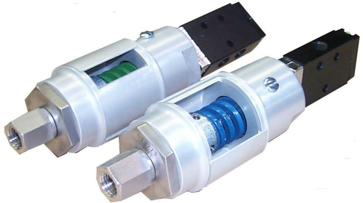
All air pilot switches are subject to deadband conditions, which should be considered when using the valve. A deadband is described as the difference in pressure between a set point of sensing pressure and a pressure at which the air valve returns to the original position. Deadband conditions vary by pressure range in percentage with higher pressure conditions reducing the deadband range.
